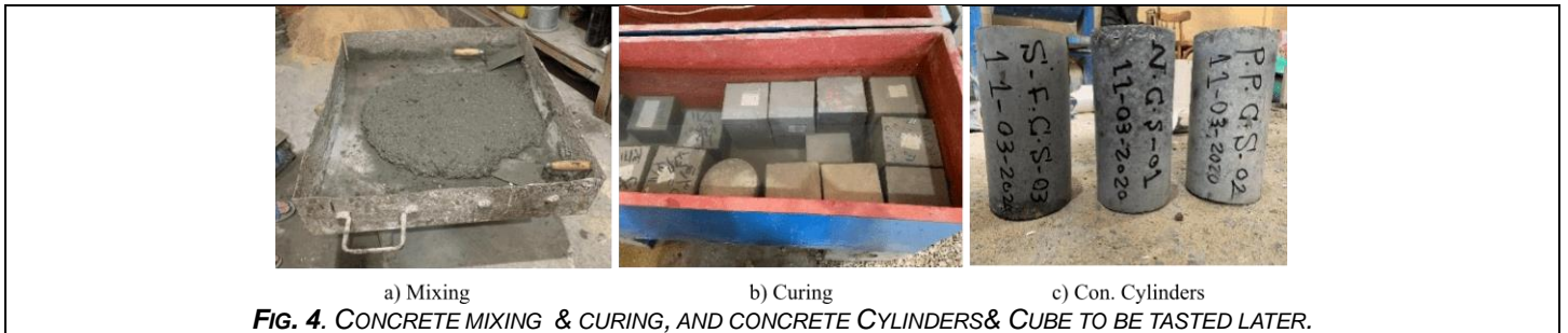
FIG. 4. CONCRETE MIXING & CURING, AND CONCRETE CYLINDERS & CUBE TO BE TASTED LATER.
